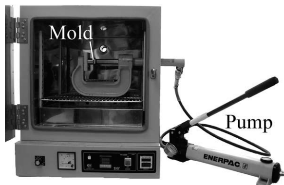
Figure 1. Photo of the setup for compression molding of the antibiotic pellets and disks.
